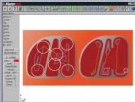
Automated pocket remachining with a smaller tool
