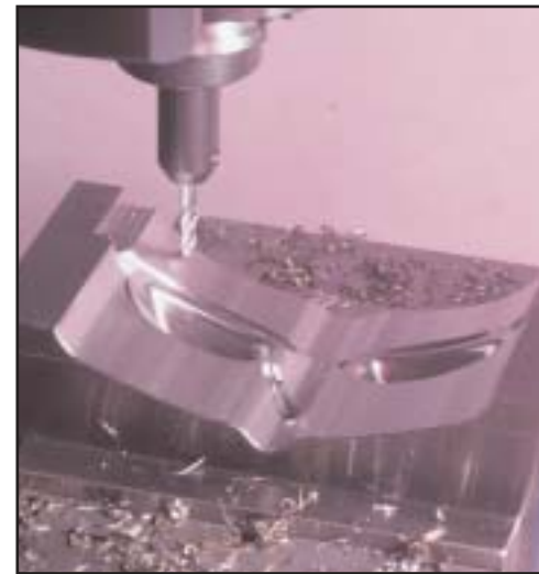
Smart Cornering - Based on the part and machine tool characteristics, Mastercam adjusts the feed rate around corners and small radii for smooth transition in tight areas.
