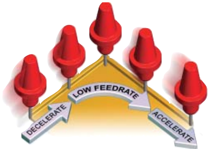
Smart Cornering - Based on the part and machine tool characteristics, Mastercam adjusts the feed rate around corners and small radii for smooth transition in tight areas.
